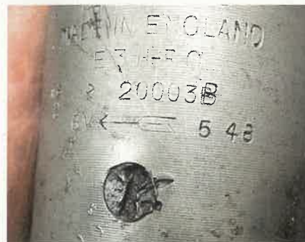
6 If all's well, the dynamo will spin or 'motor' – and in the direction of the arrow on the body/drive from the engine. If it goes the wrong way, swap 'D' and Earth brush connections.
