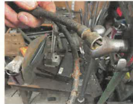
15 Next: the speedo cable; the cloth binding has frayed, but it's an original and it's not broken, so I was loath to replace it. Maybe I could smarten it up...
