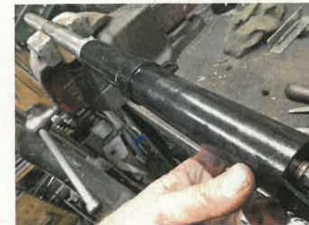
11 To test fork bushes you need to set them up at about mid position; at full extent they're close together and will feel worse than they are; the 3T's need replacing.
