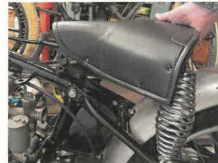
10 Lightweight BSA Bantam-size repro saddle suits the trials styling, but no surprise it's too short and the nose bracket is too narrow for the frame lug.
