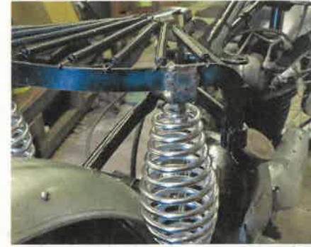
13 Cut down and reshaped, I welded them back onto the saddle frame, keeping it level and true to the bike (although the level can be adjusted with spacers).
