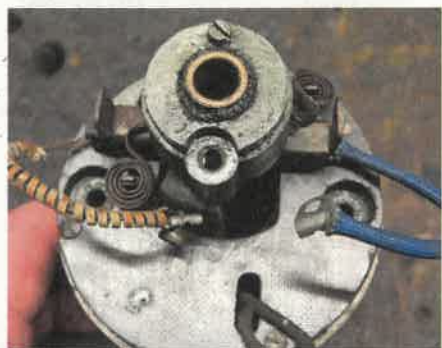
4 Of the two brushes, one goes to earth, the other to the 'D' terminal. Switching which brush OR which of the two field wires is earthed will reverse direction of rotation.
