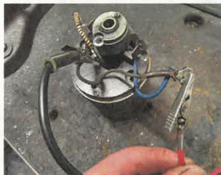
5 To test a dynamo, join the 'F' and 'D' wires together and to one battery lead, with the other lead to earth – ie the dynamo body, matching the earth polarity of the bike's system.
