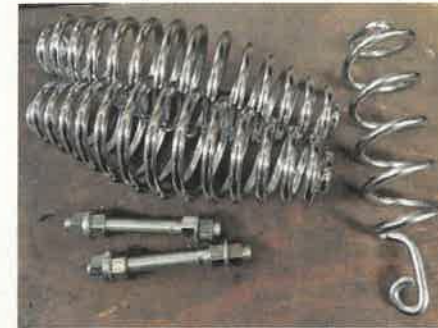
11 And it comes with corkscrews for springs! This LF Harris-made repro set was well worth £50 – looks right, fits properly, good quality and comes with fitting studs.
