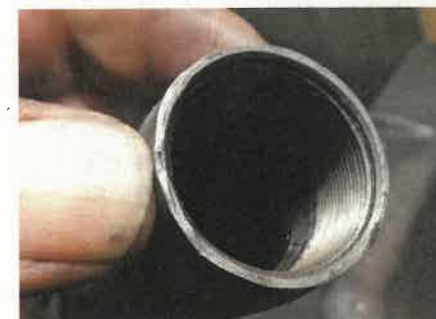
10 Back home, one fork legs wouldn't pull fully up into the yoke. It was just a sight burr where the top had been hammer-bruised sometime; it was easily filed off.
