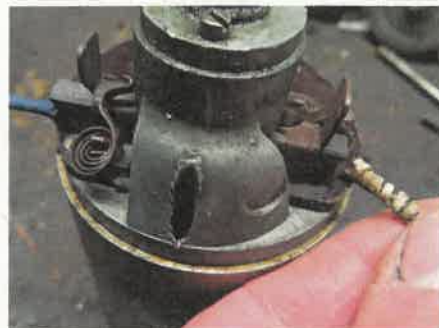
2 Two opposing carbon brushes pick up the current from a segmented copper commutator. AC current is automatically rectified into DC, ready to charge the battery.
