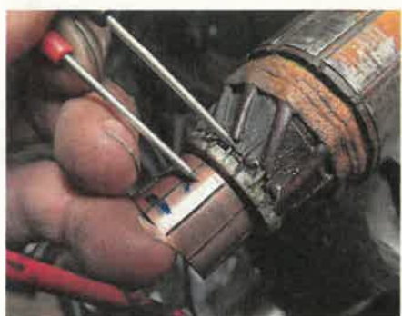
8 High resistance or 'open circuit' between segments could mean a dry solder joint between a coil wire and a segment. Poke through insulation if necessary to check.
