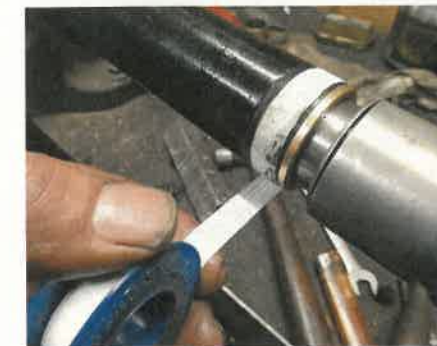
17 Before finally fitting the seal holder, use sealant or a few turns of PTFE tape on the threads; otherwise you can get a slight oil leak from here.
