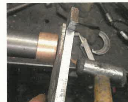
16 Bottom bush fits tightly. Vee angle aluminium makes a good removal drift; flat alloy plate makes it easier to check bush is going on squarely when fitting.
