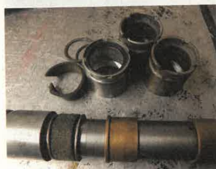
4 Felt fork seals are standard; the oil level's a fair way below the seal, but Pete bored out the new holders I supplied to take belt 'n' braces oil seals, too.
