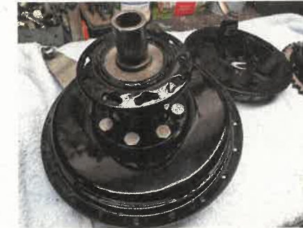
9 Here are the hubs, stripped cleaned and painted. I've got spokes on order – galvanised as standard, I think stainless would clash with the enamelled rims.
