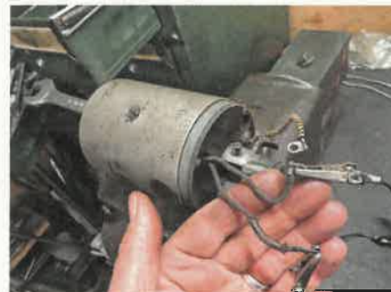
3 The two field coil wires – one goes to the 'F' terminal, the other to earth. Test-connected to a battery, the magnet should take a firm hold of a spanner.
