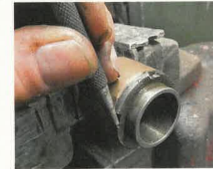
15 The castellated nut that holds the bottom bush is usually very tight; breaking the grip with careful use of a punch can be safer than using a C-spanner.
