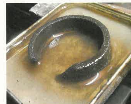
13 Any pitting can be rubbed smooth with sandpaper and won't destroy seals – especially these felt seals. Soaking in melted tallow keeps the seals oil-tight.
