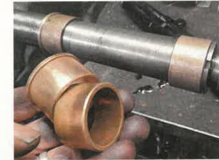
12 Fortunately, Triumph used the same bushes for years and I had a new set in my spares. The fork tubes were in good enough condition to keep.
