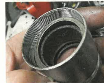
14 Steel washers sit either side of the felt seal. The lower one bears on the top fork bush, keeping it in place, so check it screws fully down before fitting fork tube.
