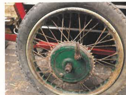
7 Next job for Pete was the wheels. The plating on the original rims is too far gone to clean up, but we might get them powder coated and then rebuild them with new spokes...
