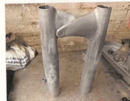
5 Original fork shrouds will go back on; they give much better protection than gaiters. After dipping, filling and rubbing down, here they sit ready for a spray coat of gloss black.
