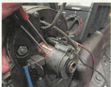
7 If it doesn't motor, check for continuity between each commutator segment – but none from any segment to the steel armature parts, meaning it's shorting to earth.
