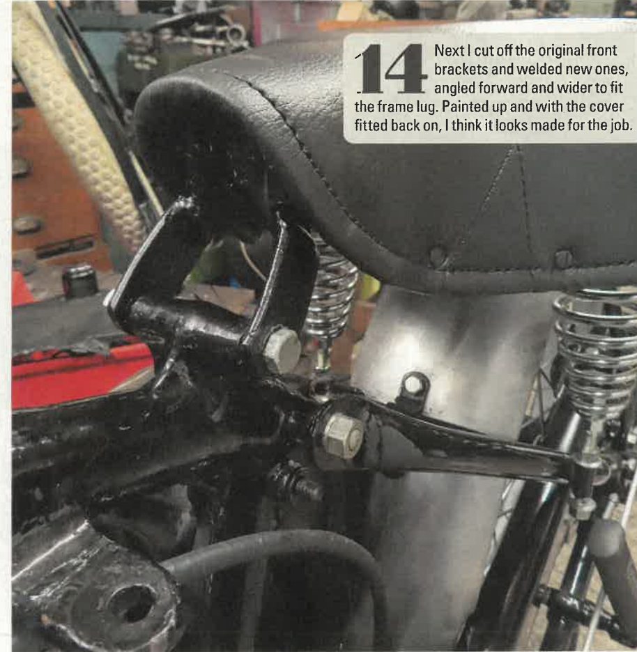
11 And it comes with corkscrews for springs! This LF Harris-made repro set was well worth £50 – looks right, fits properly, good quality and comes with fitting studs.
