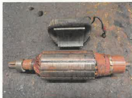
1 Dynamos produce AC current when the armature (wire coil) is rotated within a magnetic field from the field coil (an electromagnet, energised from the voltage regulator).
