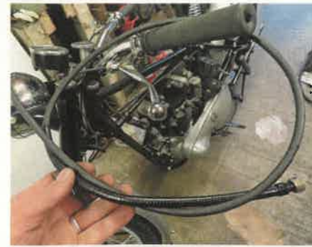
16 Job done. I was able to remove one end without damaging it, enabling me to slide some heatshrink over the original frayed binding. Good as new; well, nearly.
