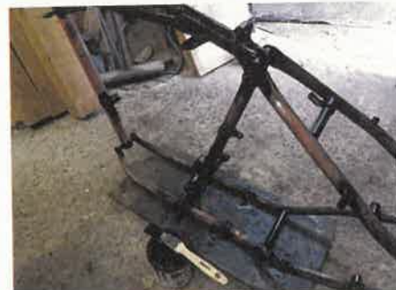
2 Paint is inky black 'International' yacht enamel. Pete recommends doing all the fiddly bits first, where runs are often generated, filling in straight tube sections after.
