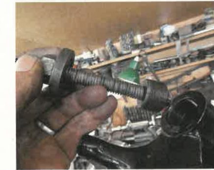
18 Fork tool pulls forks into the yoke. Ensure peg on base of the damper units, which locates in a hole in the slider, is engaged before tightening retaining bolt.
